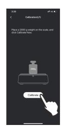
Place a 2000g weight on the scale, and click Calibrate now. (you need to get the 2000g standard weight prepared for calibration)
